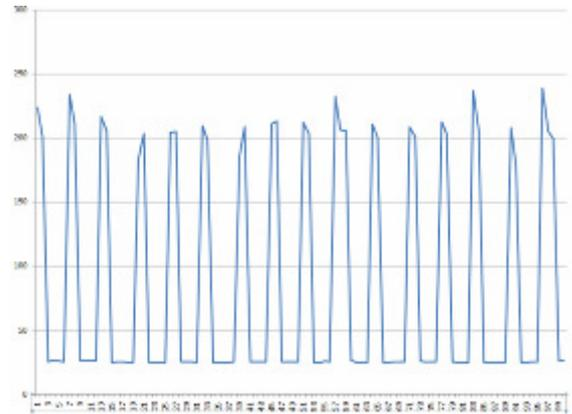
Example energy consumption of a refrigeration unit
